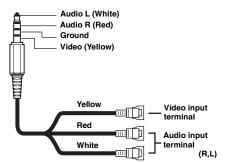
Configuration commercially available 4-pole mini AV plugs is not standardized.
