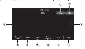
① [ \_ [ ] Calls up the Display Setup screen. (See "Display Setup Operation" on page 18)
