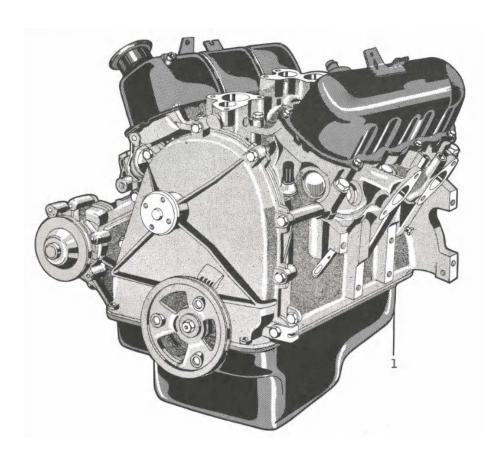
1] 122 CID six-cylinder engine (for illustration only; not installed in the Saab Sonett)
