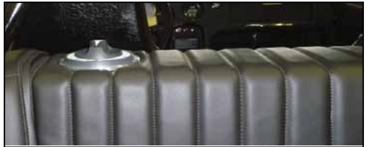
Master switch on bulkhead.
