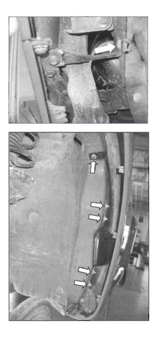
Reinstall bolt -arrow- from front inside fender well and torque to 6 Nm (53 lb-in)
